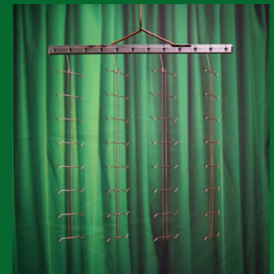
Using 45° angled hooks enables denser hanging.
